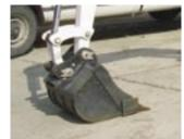
Make sure attachment is securely fastened to excavator. Check that X-Change<sup>®</sup> system (if equipped) is securely engaged.
