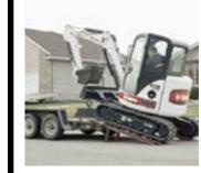
Always drive up the ramp with heavy end uphill (boom, dipper, etc.). Engage swing lock and
